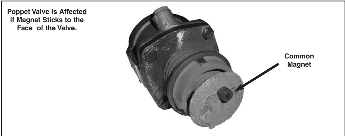
Figure 4 - Poppet Valve Magnet Check
