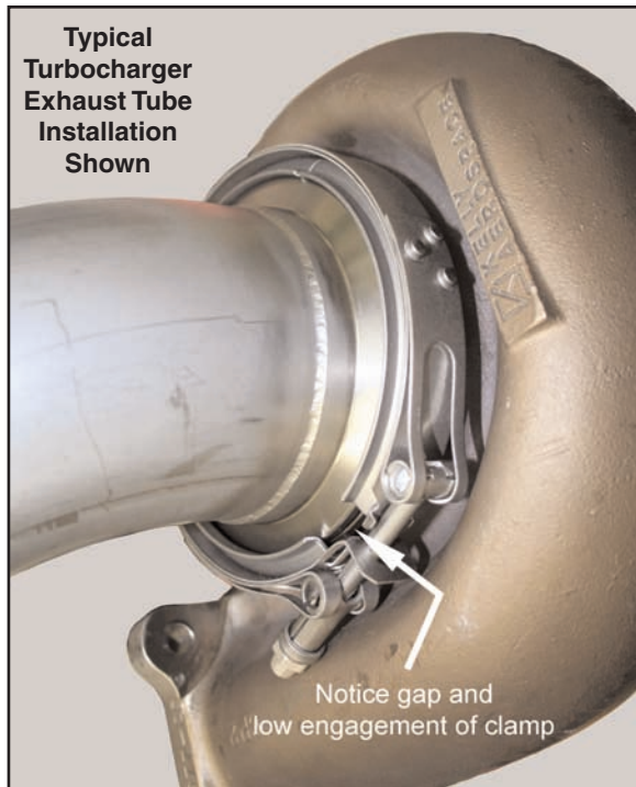
Figure 2 - "V" band Clamp Showing Gap
