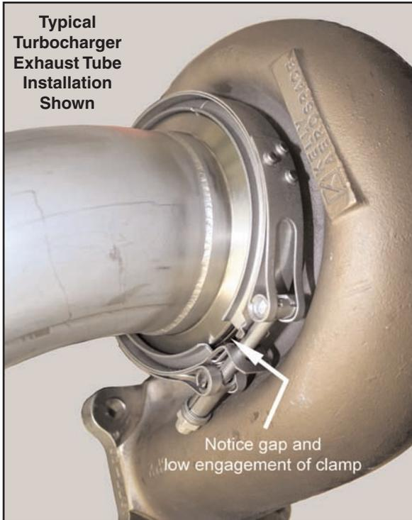
**Figure 1 - "V" band Clamp Showing Gap**
