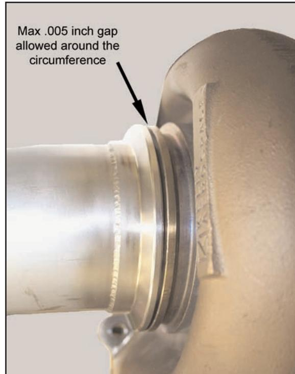
**Figure 2 - Gap Inspection Area**
